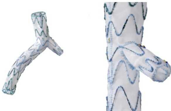
Figure 21. Photograph of the unsheathed E-liac stent graft system. The nitinol skeleton is covered by woven polyester, which is sutured with braided polyester. The asymmetric tip-to-tip spring configuration allows good conformability to the vessel's shape, which minimizes the risk of kinking in angulated anatomies while maintaining appropriate longitudinal stiffness. (Courtesy Jotec GmbH, Hechingen, Germany.) Figure and explanations taken from Mylonas et al. (151)
