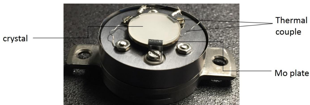
Figure 2. 3 The structure of sample stage.
