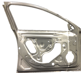
Figure 1.1: Applications of advanced high-strength steels for the mining and automotive sectors. Left: wear-resistant hoppers. Right: deep drawn car inner door.
