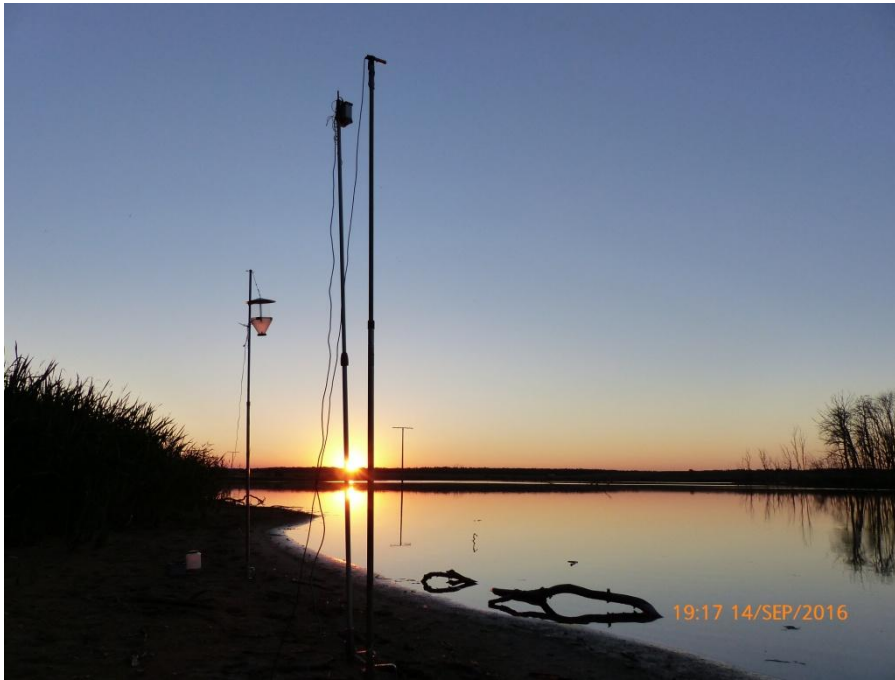
Fig. A3.1.2 Photograph of the experimental setup. The microphone was mounted on the right pole, the speaker was placed a few centimetres in front of the microphone (middle pole). The insect trap was about five metres apart from microphone and speaker, on the left pole.
