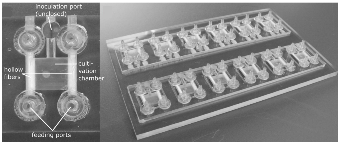
Figure 1: Miniaturized perfusion reactor. Left: Composition of a single reactor (chamber 7x9 mm). Right: Two slides with six reaction chambers in parallel each in a multititerl plate dimensioned holder.
