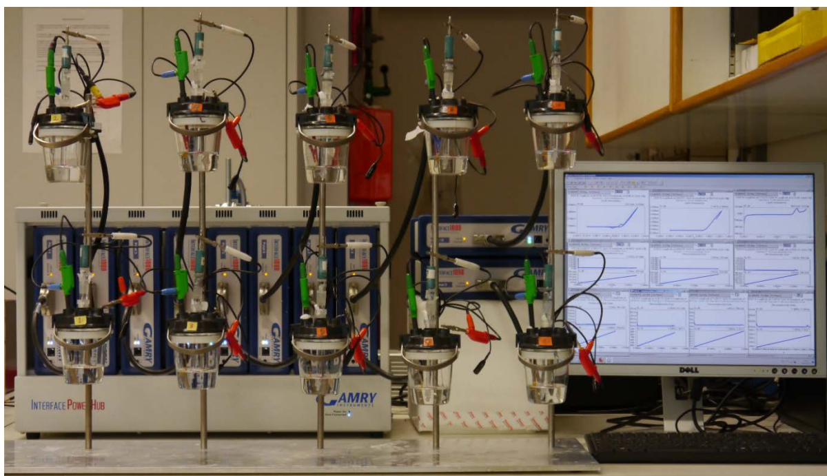
Figure 2.1. Ten parallel Gamry potentiostats (Gamry Interface 1000™, Warminster, USA) for electrochemical experiments (deposition and operation) control ten single-compartment electrochemical cells with each three electrodes.
