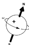
figure 1-1 – In an external magnetic field, each nucleus in a molecule can have two possible orientations: parallel or antiparallel to the external magnetic field B_0 . In a quantum mechanical
