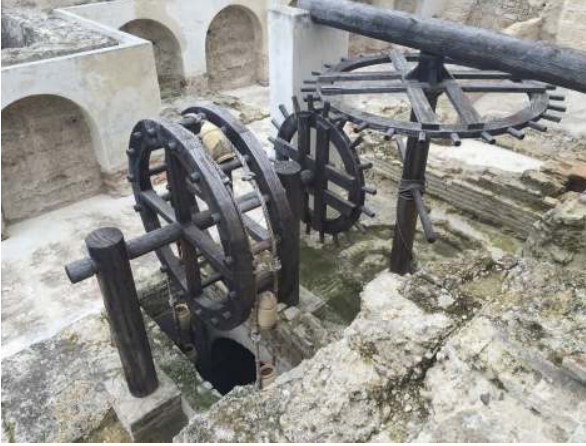
Fig. 5 A reconstructed medieval sāqiya example from Alcázar of Córdoba. This machine was powered by manpower to lift water from the cistern below, and was used to irrigate the garden.
