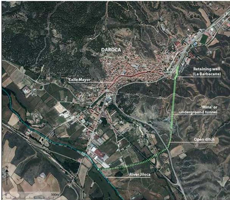
Fig. 7 The 'mine' at Daroca (Zaragoza), built in 1555–1560 to collect and drive floodwater safely away from the town.
