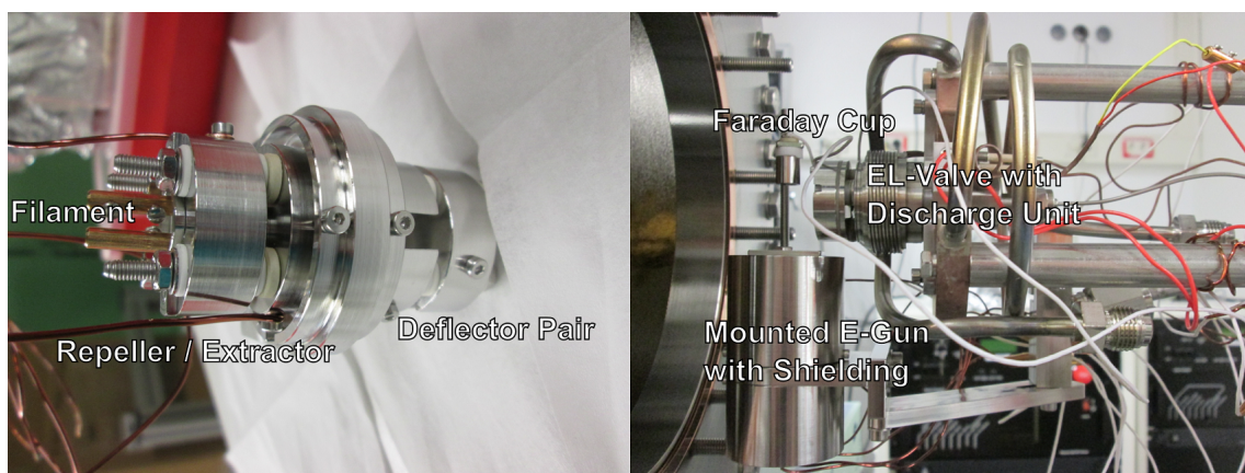
Figure 5.6.: Left: Photograph of the electron gun without the shielding. Right: Electron gun mounted in the chamber including the valve.
