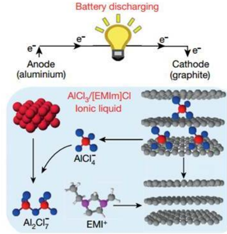
Figure 3: Schematic of Al-ion battery using graphite cathode and AlCl_3/[EMIm]Cl ionic liquid electrolyte [86].
