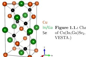
In/Ga Figure 1.1.: Chalcopyrite crystal structure Se of Cu(In,Ga)Se<sub>2</sub>. (Schematic created with VESTA.)
