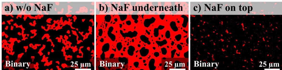
**Figure C.5.:** Binary images after heating with 0.01°C/s up to 580°C of a multilayer precursor a) without NaF, b) with 30 nm NaF under precursor and c) with 30 nm NaF on top of precursor, processed from Mo intensity distribution images (elemental images Fig. 3.5) by method of N. Otsu (1979). Dewetting determined from the binary images is a) 30%, b) 65% and c) 4% (Tab. 3.3).
