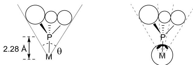
Figure 53. Tolman's definition of the cone angle (left), White's definition of the solid angle (right).
