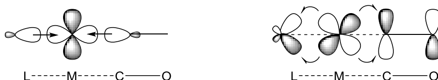
Figure 55. \sigma -donation (left) and \pi -back donation (right) contributions to the M-L bond in a M-CO complex.
