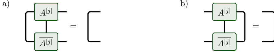
Figure 3.4. – Illustration of the condition on the component A^{[j]} of an MPS for being left normalized (shown in a)) and right normalized (shown in b)).
