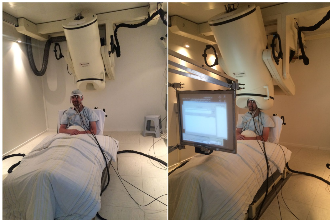
Figure 1. Multimodal setup in MEG environment. In the pictures, the black cables with fibre optics based sensors attached on the body and head are optical fibres for measurements of cNIBP and NIRS. On the right, shown is performing of simultaneous recording with the setup. During imaging, the display is used to instruct the subject to perform the given task.
