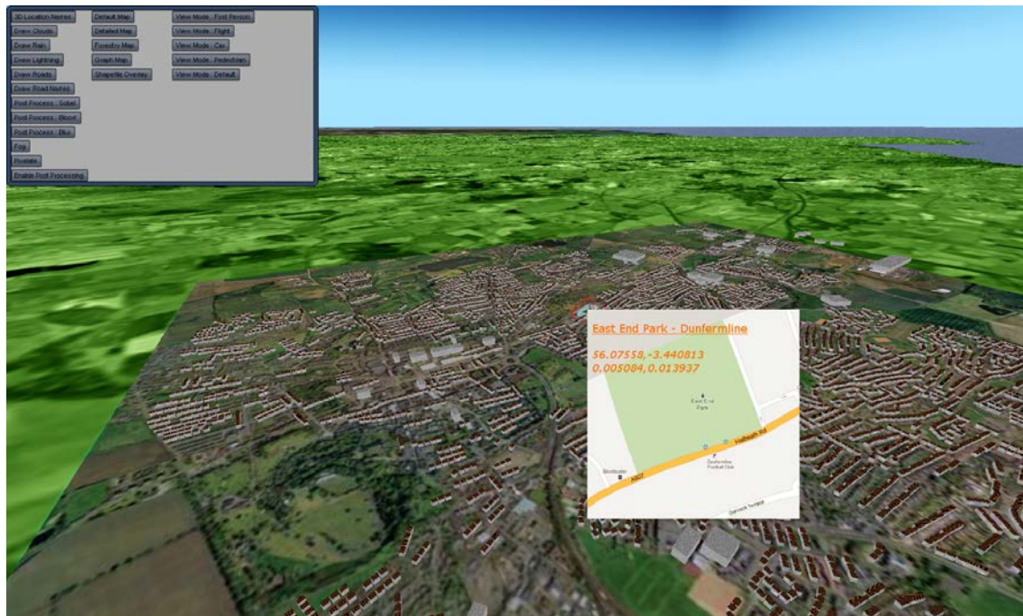
Figure 7: LEX Showing aggregation of different data sources: Aerial Photography, Google Maps and USGS Digital Terrain Models
