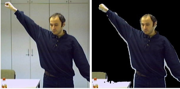
Figure 7. Left: The scene as captured by the 2D-camera. Right: The segmentation by depth range check after calibration. The extra pixel layer around the teacher is actually two or three pixels wide. The table is also recognized as foreground because it lies in the same depth interval.
