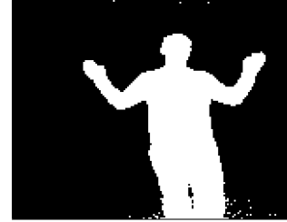
Figure 11: The mask obtained by depth range check for segmenting an instructor, as computed by us using a 3D camera.
