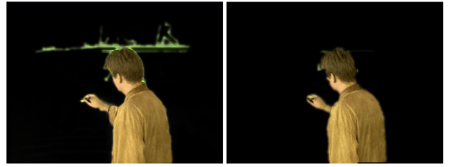
Figure 6: The result of board stroke suppression. Left image: without suppression; right image: with suppression.
