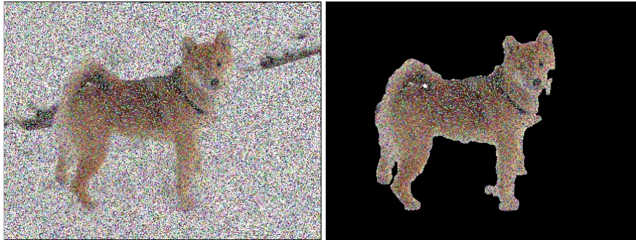
Fig. 9. A fairly high signal-to-noise ratio has only little effect on the segmentation (left: original image, right: segmented dog).
