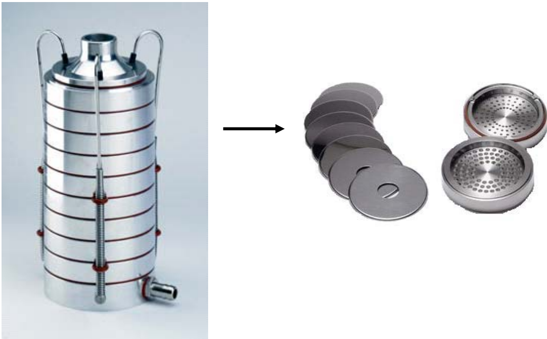
Figure 3-13: Photograph of the assembled 8-stage Andersen Cascade Impactor (ACI-8). On the right side, a view of the individual components: separation stages and collection plates.
