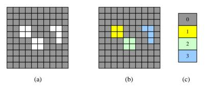
Figure 16. a) binary original Image, b) Resulting image of the operation bwlabel Considering as connectivity connection-4 and (c) the color code.
