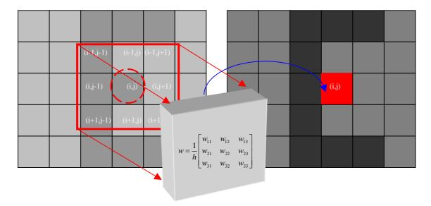
Figure 8. Spatial filtering for one mask of 3 x 3.
