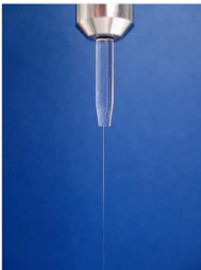
Figure 3.7. A quartz capillary nozzle with filament of water
