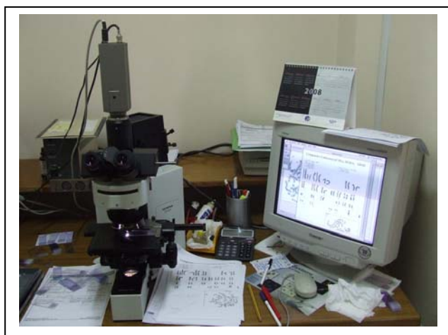
Figure 2: A Vysis system composed of BX50 Olympus microscope, CCD camera and karyotype software. Cytogenetic laboratory, CPHL, MoH, Oman
