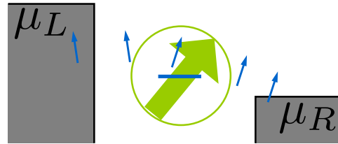
Figure 5.1. Sketch of the single-molecule junction. The electronic spins interact with the localized magnetic moment.
