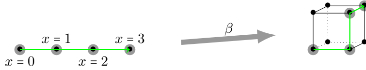
Figure 7.2: The four states of a single variable x \in \mathbb{M}_4 and its image under the map \beta onto the cube of the three Boolean variables [x \geq 1] , [x \geq 2] , [x \geq 3] on the x, y, z -axis. Elements outside the image of \beta are contradictory assignments as e.g. [x \geq 1] \cdot [x \geq 2] \cdot [x \geq 3] , corresponding to the front-left-top vertex.
