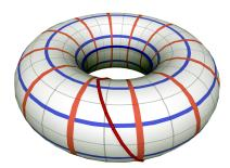
FIGURE 2.2: Once the curl free field  $\hat{X}$  is found by Hodge decomposition, an initial parameterization can be computed by integrating  $\hat{X}$ . However, parameter lines are discontinuous unless integral periods of the two dual cycles are assured.
