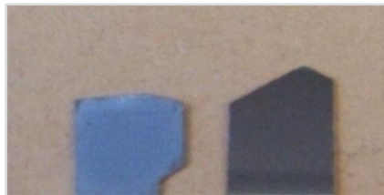
Figure 3.15: Photograph of the powdery film on Si substrate (left) and the bare Si wafer (right).
