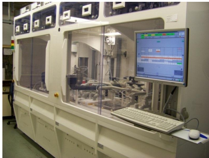
Figure 2.9: Schematic (top) and photograph (bottom) of an ILGAR in-line prototype coater for substrate up to 30 \times 30 \text{ cm}^2 designed by SINGULUS STANGL Solar in collaboration with Helmholtz Zentrum Berlin [70].
