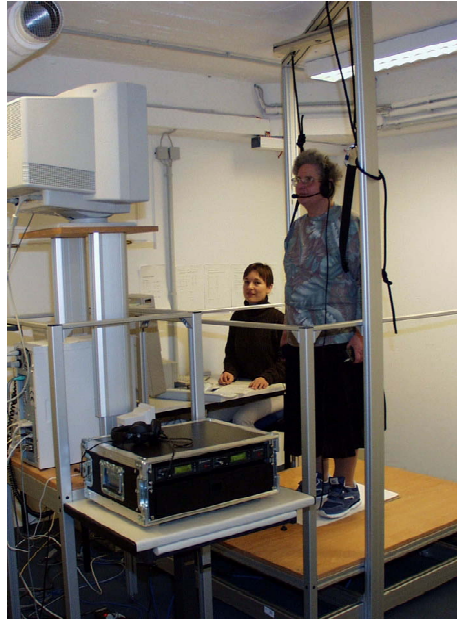
Figure 8. The experimental setup showing an older adult performing a dual task: The person listens to the acoustically presented stimuli and presses buttons while keeping balance on the movable force platform
