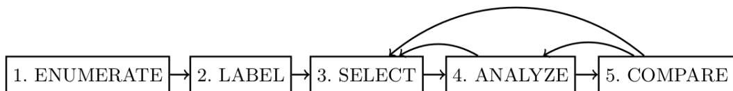
Fig. 2.5. Workflow implemented in Tremppi (picture taken from [90]), with a five step process for enumerating, labeling, selecting, analyzing and comparing models in the model pool.
