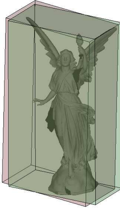
Figure 6.6: Lucy: 262909 vertices, 525814 triangles, 622 convex hull vertices, 1240 convex hull triangles and two different PCA bounding boxes - the green box is obtained with PCA-CH and the pink box is obtained with CPCA-volume algorithm.
