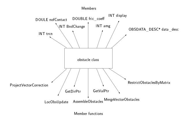
Figure 4.1: Obstacle problem class and member functions
