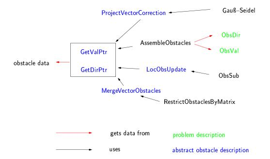
Figure 4.2: Relations between the member functions of the obstacle problem class
