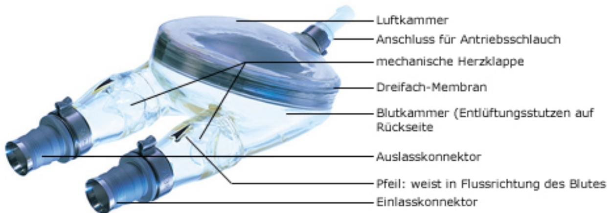
Abbildung 1: EXCOR-Pumpe <sup>11</sup>.
