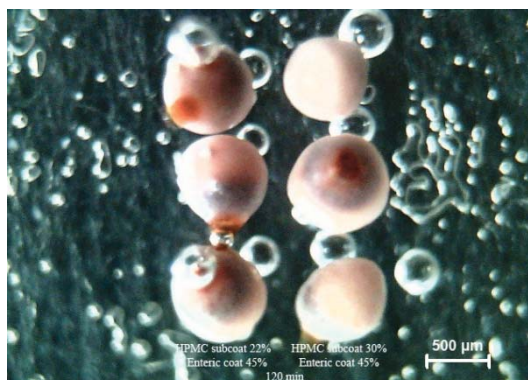
Fig. 36 Swelling of top-coated ilaprazole pellets in 0.1 N HCl: 22% vs. 30% HPMC subcoat
