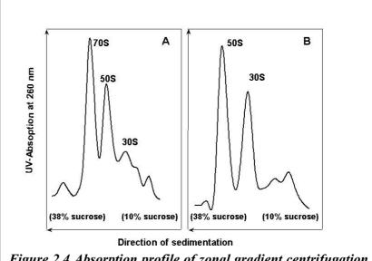
Figure 2.4 Absorption profile of zonal gradient centrifugation of Ribosomes. (A) 70S tight couples ribosomes (H20M6N30SH4) (B) 30S and 50S ribosomal subunits in dissociating conditions (H20M1N200SH4)
