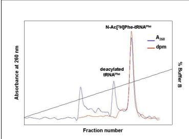
Figure 2.1 Purification of N-AcetylPhe-tRNA<sup>Phe</sup> from E. coli by reversed phase HPLC after deaminoacylation
