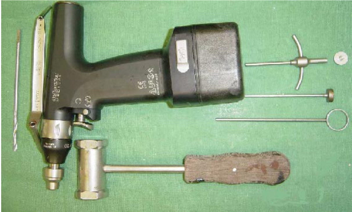
Figure 31: Showing the complete Jamshidi set for collection of cancellous bone graft.
