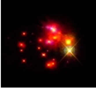
Figure 2.1.: Photograph of a multiply filamenting near-infrared terawatt laser pulse projected on a screen. Filaments show up as colorful spots of visible supercontinuum radiation (see text).
