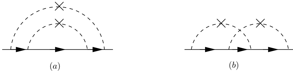
Figure D1: Diagrammatic representation of second-order contributions to the electron self-energy. In the non-crossing or self-consistent Born approximation (SCBA), only diagrams without crossing impurity lines, such as the one labeled (a), are retained, while diagrams with crossing impurity lines, such as the one labeled (b), are neglected.
