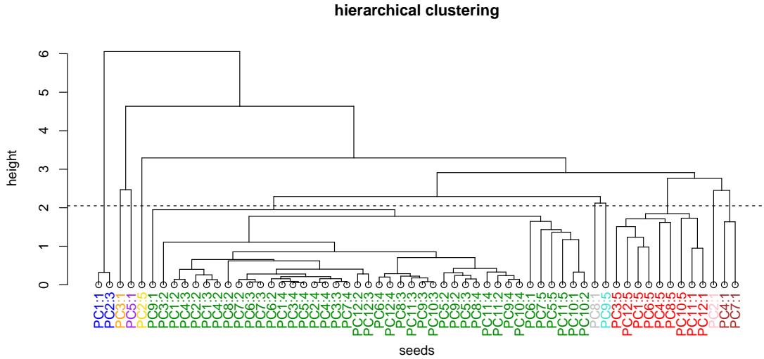
Figure 4.6: Hierarchical clustering of seeds in the initialization algorithm. A pairwise distance between seeds is computed and is used for hierarchical clustering. The agglomeration of the leaves stops when k subtrees remain disjoint, where k is the desired number of clusters to initialize. In this case k = 10 and each subtree is represented by a distinct color of the leaves. The k subtrees can be used to initialize k different negative multinomial distributions.
