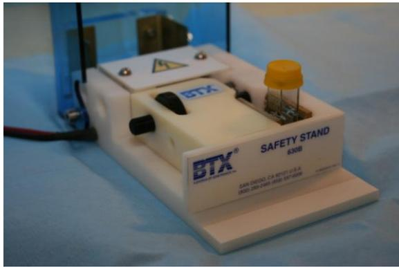
Abb.13 BTX Safety Stand 630B (Genetronics)
