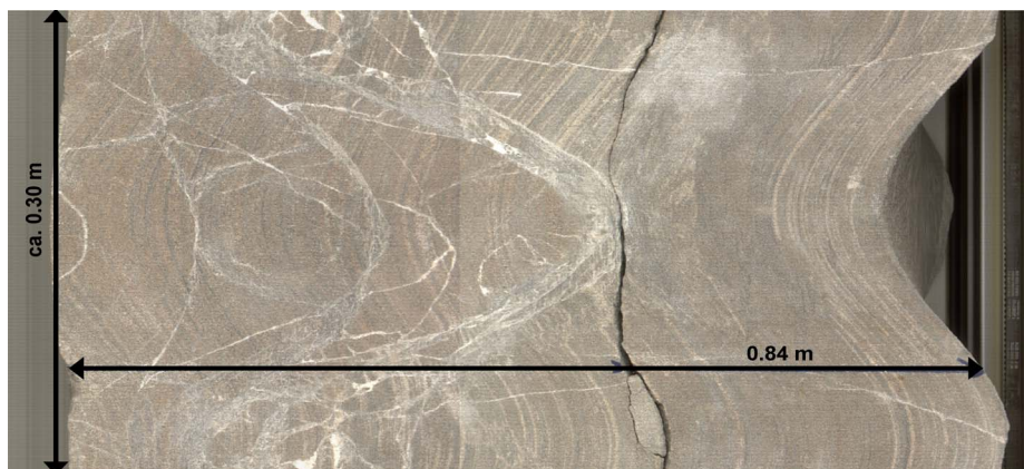
Figure 5.2: Unwrapped scan of a typical drill core of the study area, representing Rotliegend dune sandstone with sedimentary bedding (brownish) and quartz-filled fractures (whitish).
