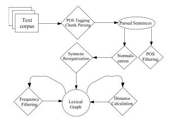
Figure 5.2: Main steps during graph construction
