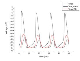
Figure 8.5: Peripheral depolarization of the B21 cell. The graphs show voltage spread in the first peripheral compartment (Vm1), in the soma (Vmsoma), and in the last lateral compartment (Vmlat10).
