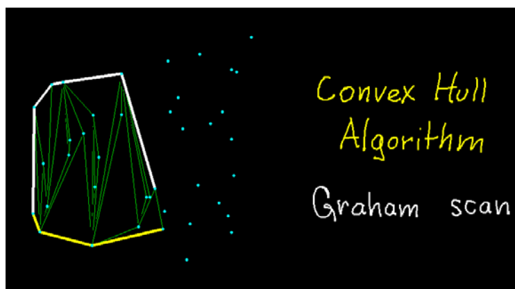
Figure 4.22 Progress of the convex hull algorithm. Lines tested and rejected are shown in green.
