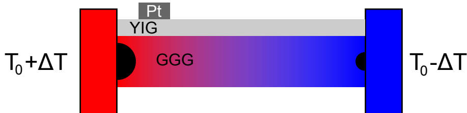
Figure 9: Schematical setup for measuring the transverse spin Seebeck effect. Two thermal heat reservoirs are attached to the gallium gadolinium garnet crystal ( \text{Gd}_3\text{Ga}_5\text{O}_{12} ). On top of the GGG crystal, there is an evaporated YIG-film, whose thickness is much smaller than the thickness of the GGG. Beyond that, there is a platinum stripe on top of the YIG-crystal. The voltage is measured on the platinum stripe perpendicular to the plane of projection. The magnons in the YIG-stripe are thermally not connected to the heat reservoirs.
