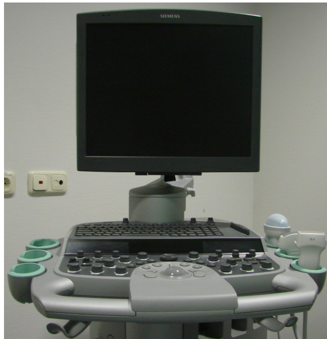
Picture 1. Siemens Acuson S 2000 ultrasound machine in an examination room in the Klinik für Geburtsmedizin at Campus Virchow Clinic. This ultrasound system was able to take video clips in relatively high frame rates without compressing the image information.
