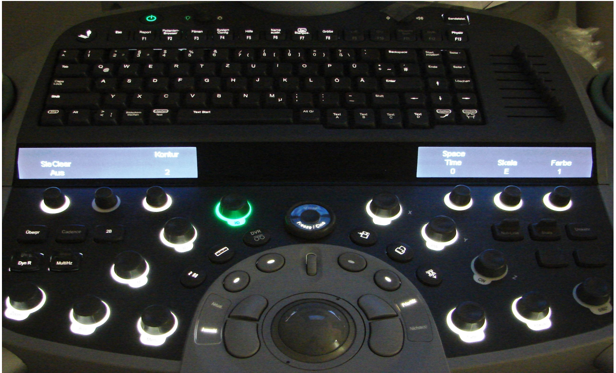
Picture 2. The console of the ultrasound system and presets recommended by the provider to capture video clips for evaluation with Velocity Vector Imaging (VVI) software. VVI is the trade name of feature tracking algorithm registered by Siemens Medical Solutions, USA.
