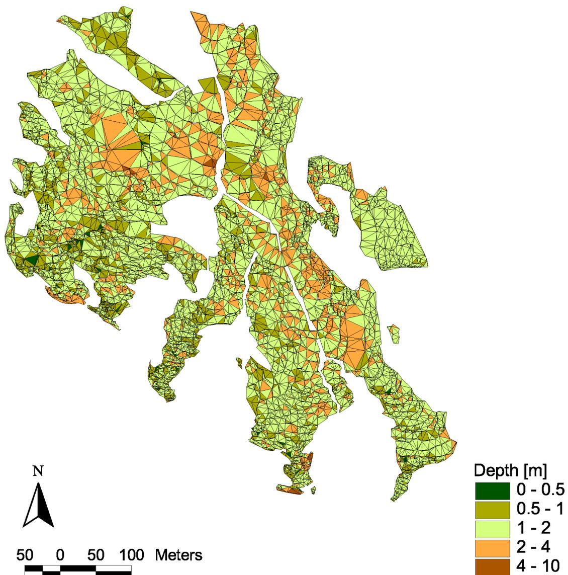
Figure 5.1 Calculated soil depth of triangle irregular network (TIN)
