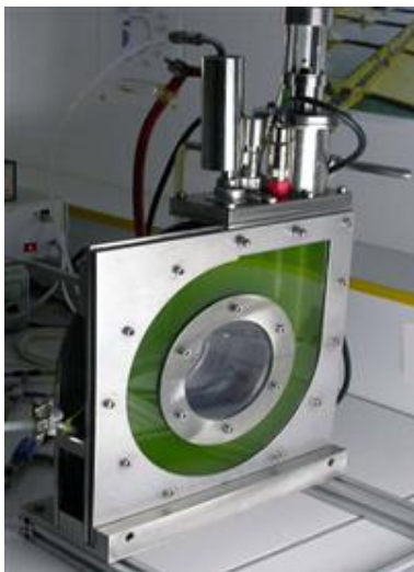
Figure 7.1: A torus photobioreactor. The figure is taken from http://www.mazenalamir.fr/ANR_CLPP/bioreacteur.html .
