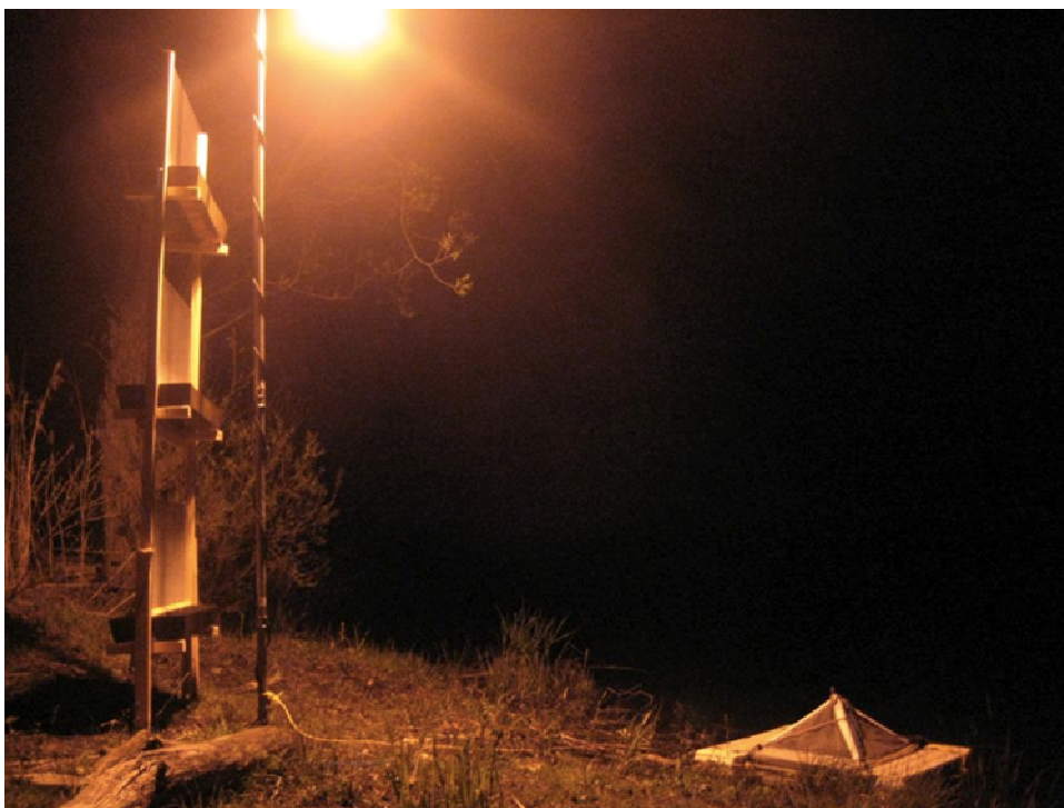
Figure 1. Flight intercept trap (location: 0 m from artificial light) with an emergence trap floating on the Spree River in front of it. Light level (lx) at each tray height written in white. Photo credit: E. K. Perkin
