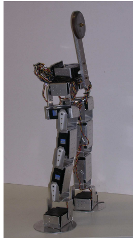
Figure 3.2: “Dany Walker V1” biped robot with inverted pendulum.
