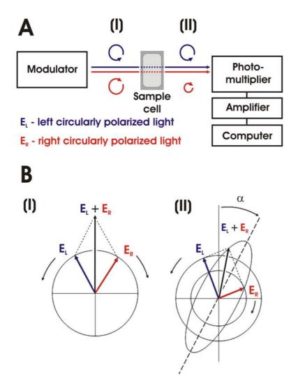
**Figure 4.1.** Instrumentation and working principle of circular dichroism. (A) Schematic chart of a two-beam CD spectrometer. (B) Field vectors of left (blue) and right (red) circularly polarized light and their superposition (black), before (I) and after (II) passage through the sample.
