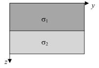
Figure 1.1: Scheme of a 1-D layered earth of conductivity  $\sigma_1$  and  $\sigma_2$ . The impedance phase  $(\varphi)$  behaviour by the diffusive process is:  $\sigma_1 < \sigma_2 \implies \varphi > \pi/4$
